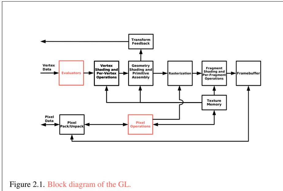
Figure 2.1. Block diagram of the GL.
