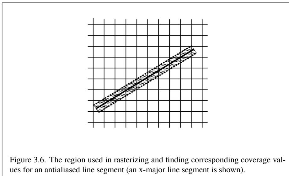
Figure 3.6. The region used in rasterizing and finding corresponding coverage values for an antialiased line segment (an x-major line segment is shown).
