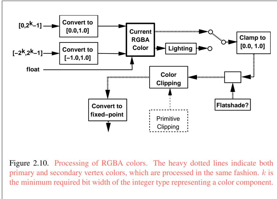
Figure 2.10. Processing of RGBA colors. The heavy dotted lines indicate both primary and secondary vertex colors, which are processed in the same fashion.  $k$  is the minimum required bit width of the integer type representing a color component.
