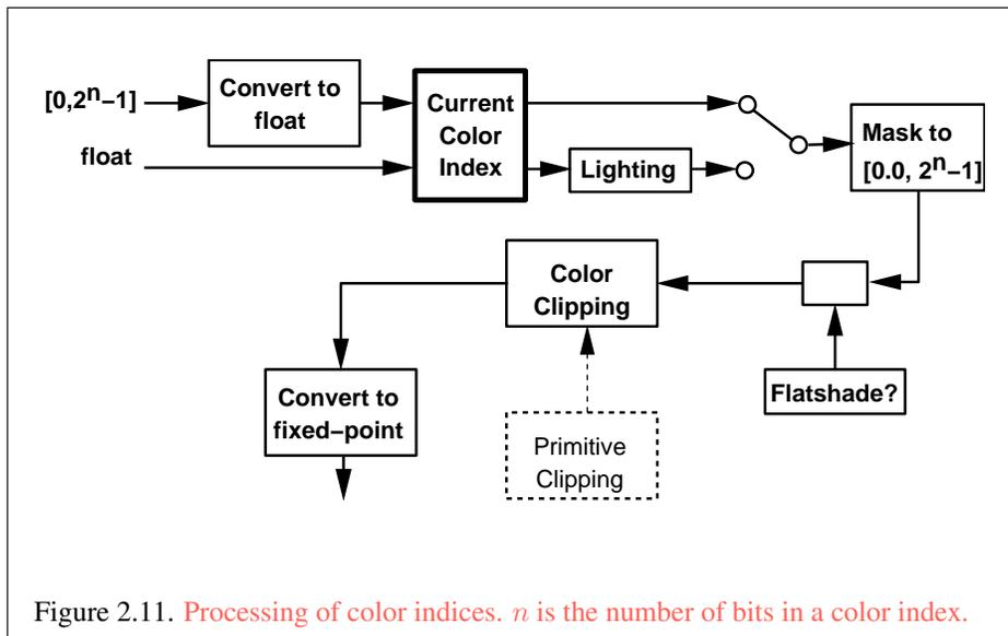
Figure 2.11. Processing of color indices.  $n$  is the number of bits in a color index.
