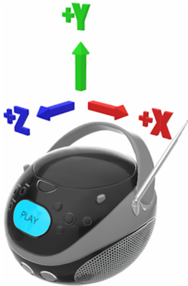
Figure 2. glTF Coordinate System Orientation
